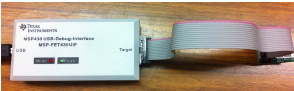
Figure 16 MSPFET430 USB Debug Interface.
